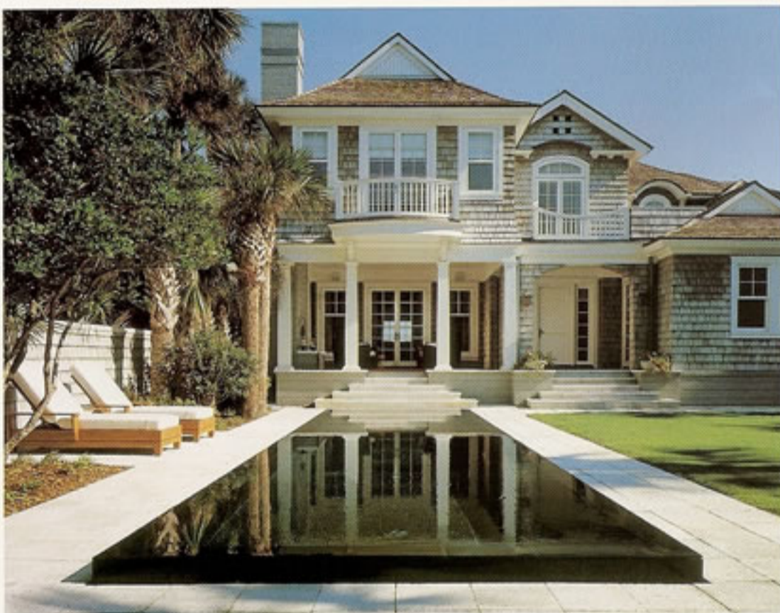
REFLECTIVE: The “elevated perimeter overflow” design serves as a reflective fountain but is also a swimming pool. The sides of this Ponte Vedra Beach pool are finished with black granite; the interior is black ceramic tile.
